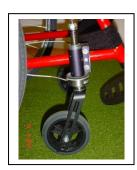
The synchronisation of the hand-rim and castor data allowed a detailed examination of how the push forces changed during a propulsion stroke, and how this relates to castor weight. By changing the axle position, and hence the tippiness of the chair, it was possible to measure the effect of stability on push stroke dynamics.
