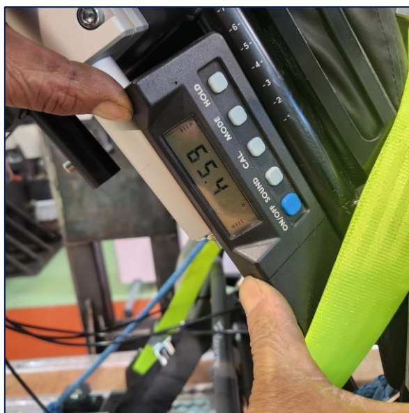
Test 2, D23-008, Back support angle set at 25° to vertical axis (90°-65.4°)
