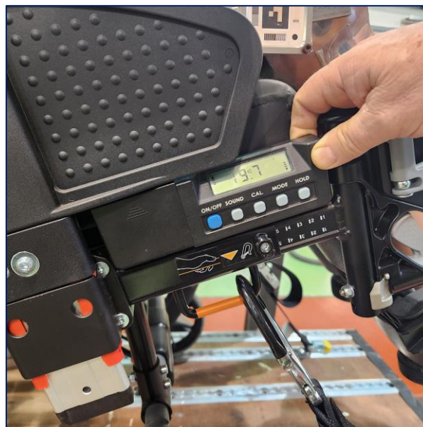
Seat rail angle set at nominal 20° to horizontal.
