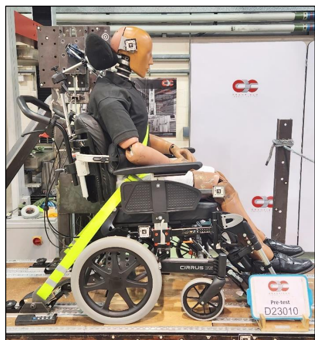
D23-010 Baseline Test, Surrogate Vehicle Anchored Occupant Restraint System Layout
