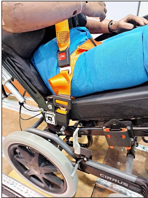
Test 3, D23-013, RH tongue and buckle arrangement, pre-test
