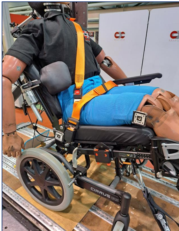
Test 3, D23-013, Front ¾ view of lap belt position on the pelvis of the ATD, post-test.
