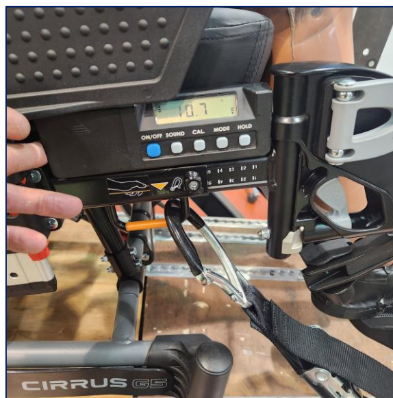
Test 2, D23-008, Seat rail set at 10° to horizontal
