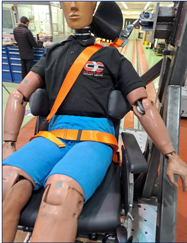
Test 3, D23-013, Front view of occupant restraint system position, post-test
