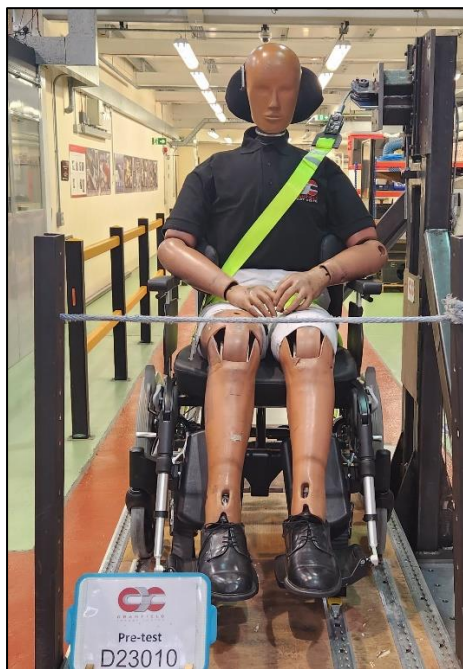
D23-010 Baseline Test, Surrogate Vehicle Anchored Occupant Restraint System Layout
