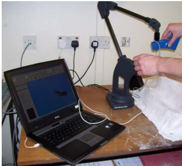
Figure 1. Microscan laser scanner: Scanning in progress
