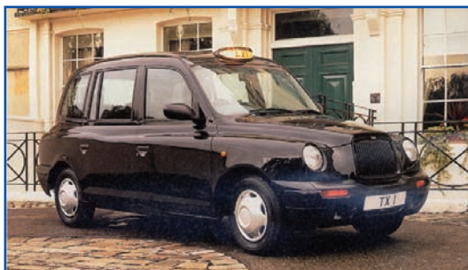
Fig. 8 – TX1 London taxi Produced by London Taxi International. Designed by Jevon Thorpe. Higher and wider, the new taxi accommodates electric wheelchairs (from the side and not from the rear!) and prams; it includes a child seat, a passenger/driver intercom, reading lights, a mirror and a plug for recharging cell phones. The door handles light up when the taxi is free, the internal handles and the edges of the seats are colour-contrasted for better perception.
