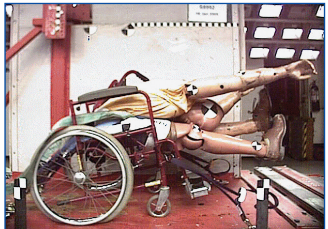
The result of not having a side wall-anchored shoulder belt anchorage
