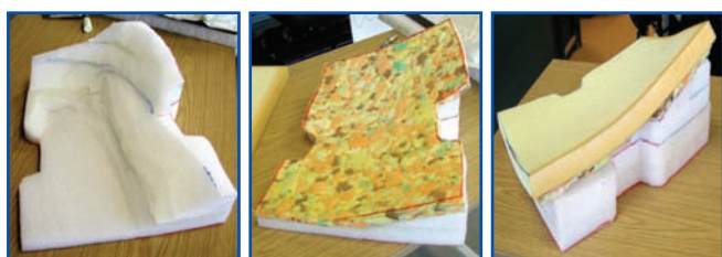
Pic. 2 – Manufacture of asymmetrical cushion.
