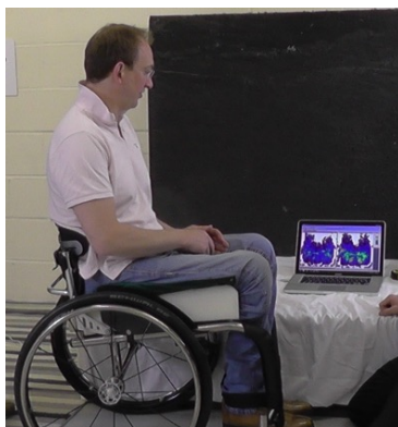
Figure 2 – Example of the pressure mapping test set up.
