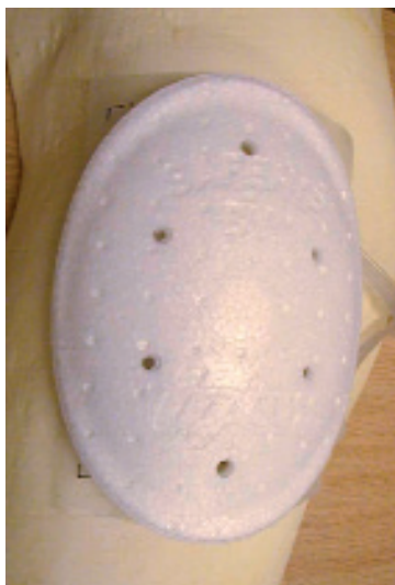
Interface pressure pad under a rigid hip protector pad
