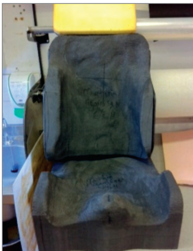
Fig 2 – Carved foam seating system with custom made dimensions
