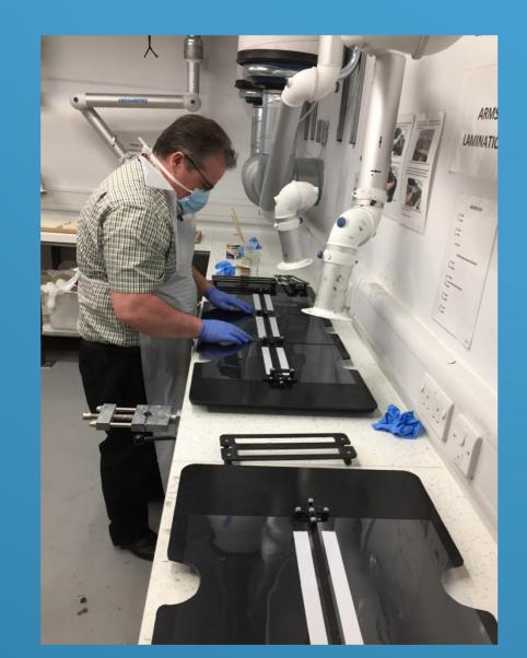
Jigs were produced to ensure continuity of product, for gluing the foam and acetate and cutting of elastic.
