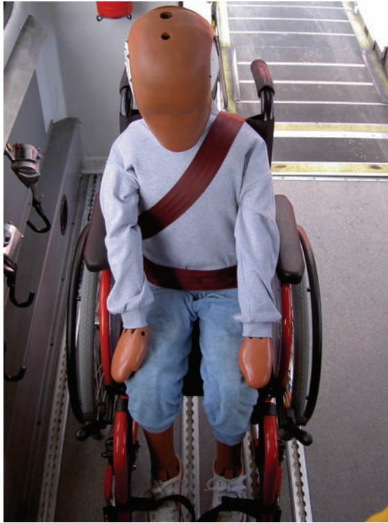
Figure B5 Seat belt geometry in a typical M2 vehicle with a flexible wheelchair space
