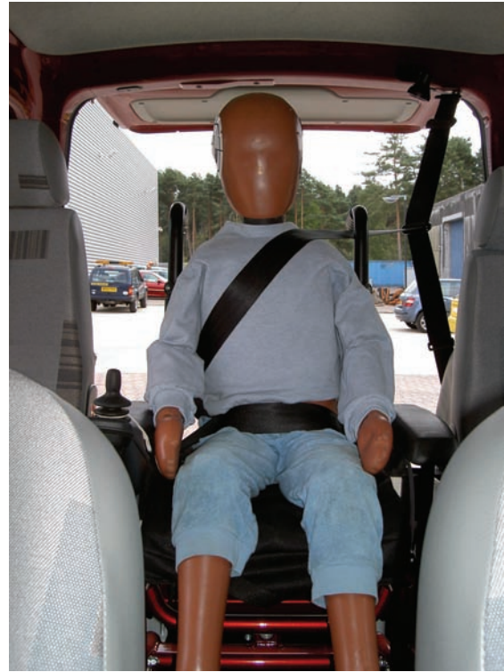
Figure B4 Lap belt anchorage location in an M1 vehicle with a permanent wheelchair space and the effect on belt path
