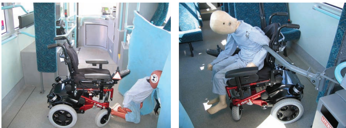
Figure 44 Ejection and entrapment of child dummies observed in testing with horizontal rail
