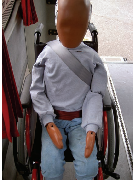
Figure B13 Seat belt geometry with a manual wheelchair in a coach
