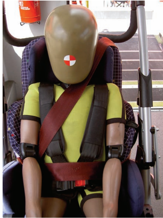
Figure B5 Seat belt geometry in a typical M2 vehicle with a flexible wheelchair space
