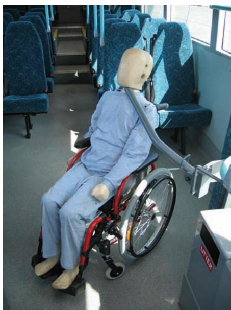
Figure 45 Horizontal rail rose during testing, resulting in contact with child dummy's chest and neck
