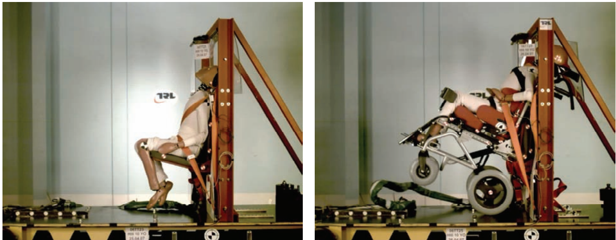
Figure 33 Neck extension in selected tests with ten year old dummy
