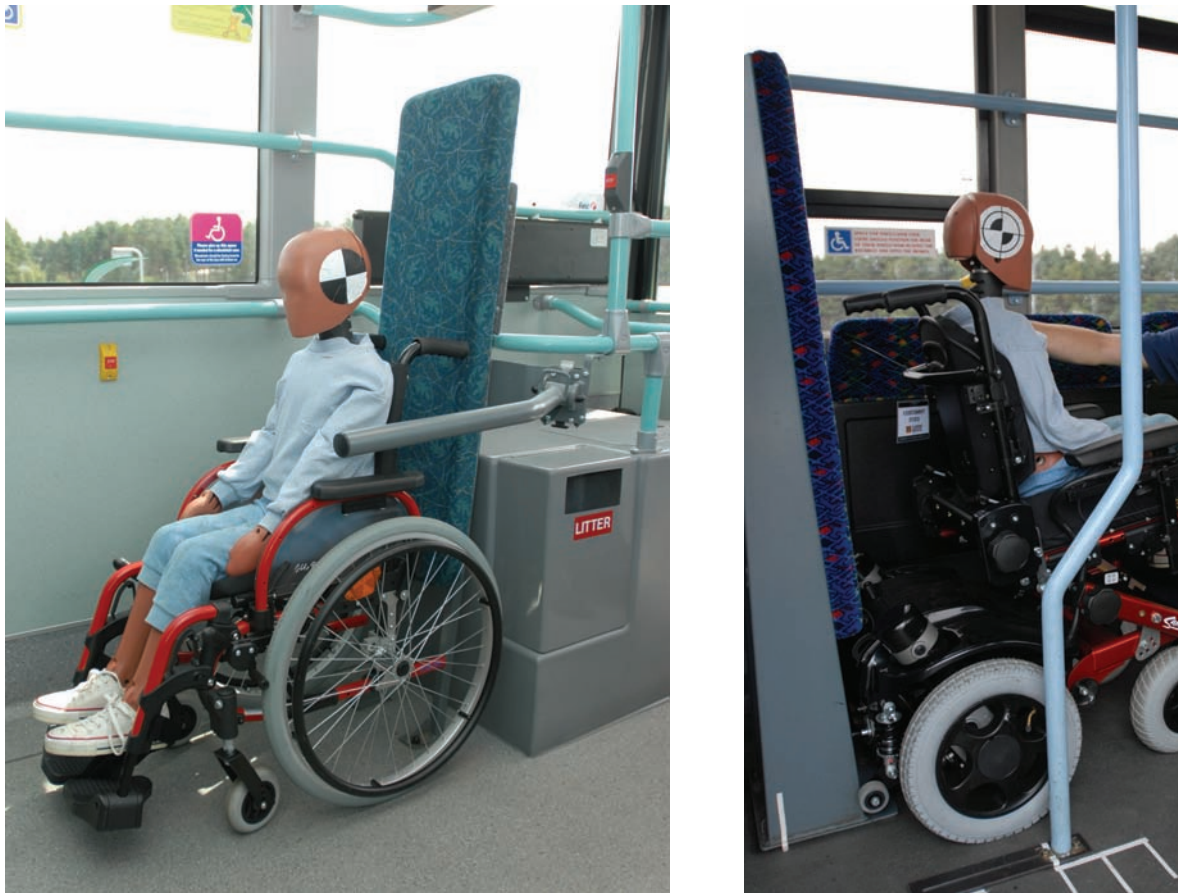
Figure B15 Wheelchair and backrest interaction in low floor buses
