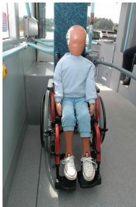
Figure 42 Example of the distance between a typical children's wheelchair and the method of restricting lateral movement in a bus
