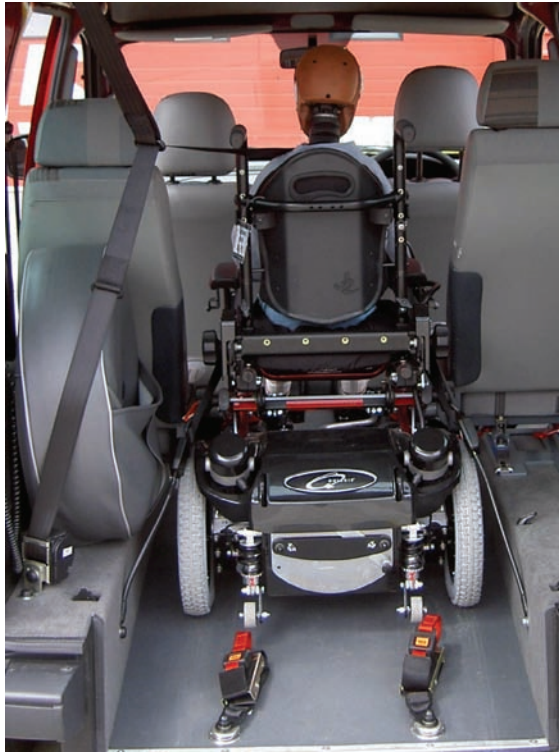
Figure B4 Lap belt anchorage location in an M1 vehicle with a permanent wheelchair space and the effect on belt path
