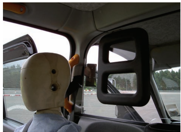
Figure B9 Proximity of head to vehicle structures in purpose built or adapted taxis
