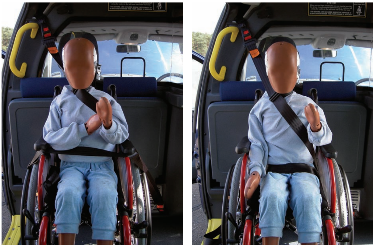
Figure B11 Seat belt geometry with a manual wheelchair in an adapted taxi
