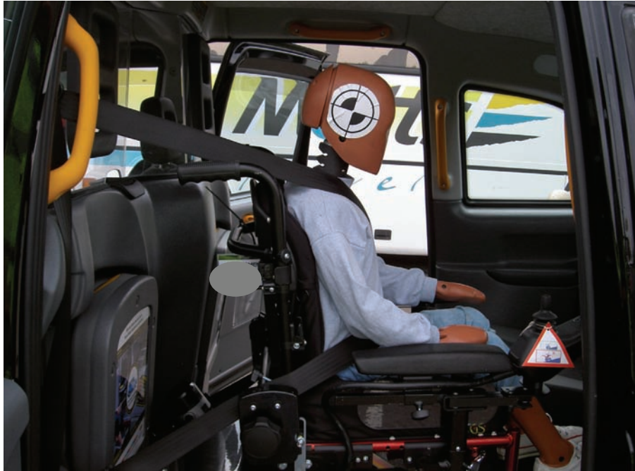
Figure B10 Example of the gap between the bulkhead and the backrest that can result in purpose built or adapted taxis
