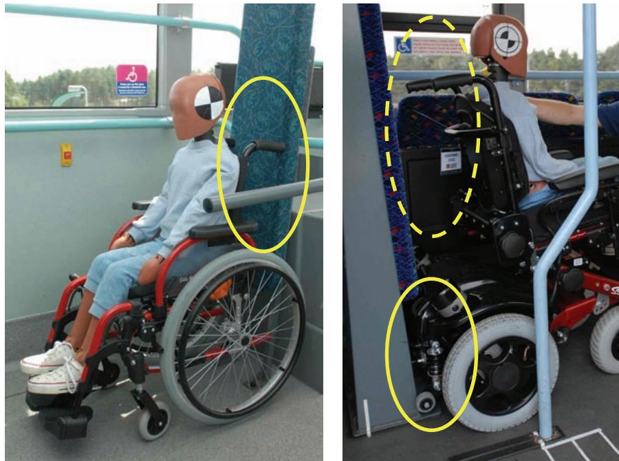
Figure 41 Examples of compatibility between children's wheelchairs and the backrests in typical buses
