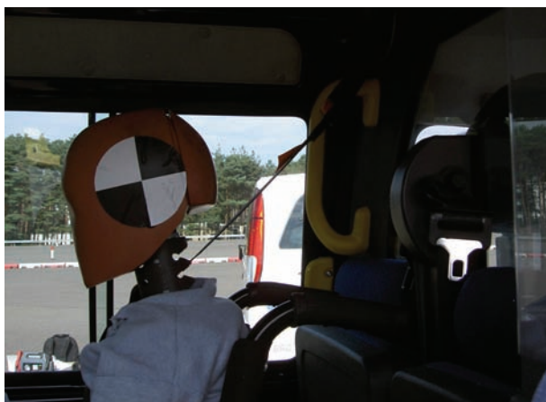
Figure B9 Proximity of head to vehicle structures in purpose built or adapted taxis
