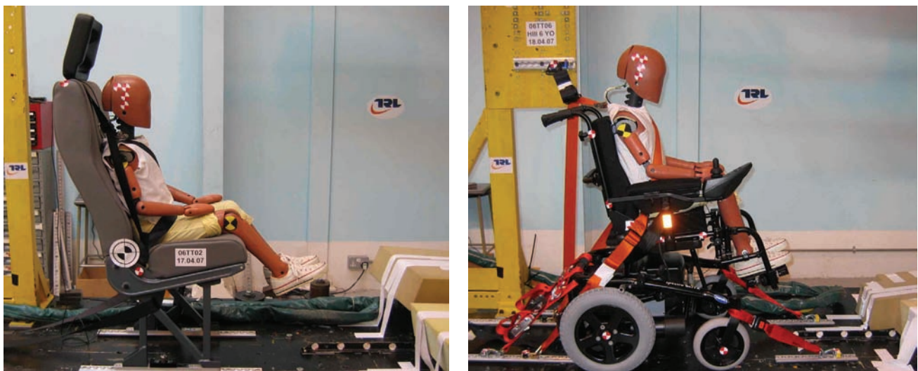
Figure 12 Forward facing six year old child dummy restrained in a vehicle seat (left) and electric wheelchair (right)
