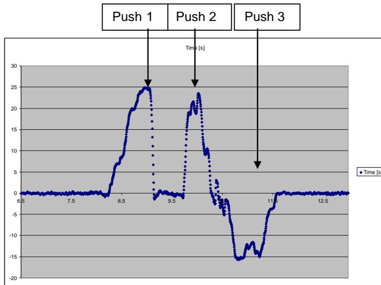
**Peak Mz** shows a significant difference ( $p = .023$ ) in **Push 1** between the tippy and stable set up with a greater Peak Mz performed to flip the castors with the wheelchair in the stable position (see **Figure 14**)
