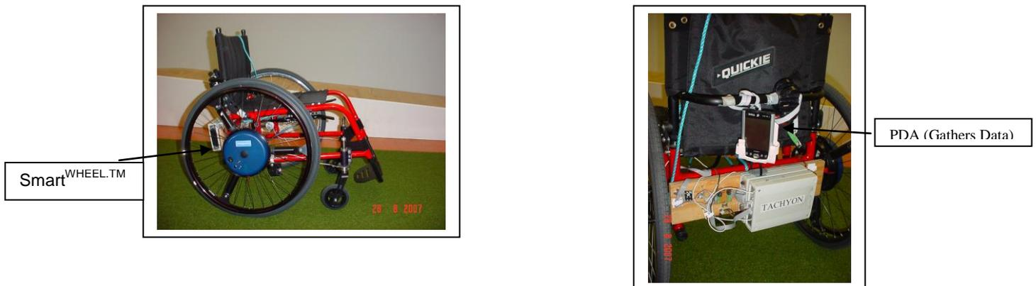
Force sensors, integral to the castors, measured weight distribution during functional mobility tasks in order to gather dynamic data (**Figure 3**). These were calibrated and validated by the research team (WOWSUP 2007).
