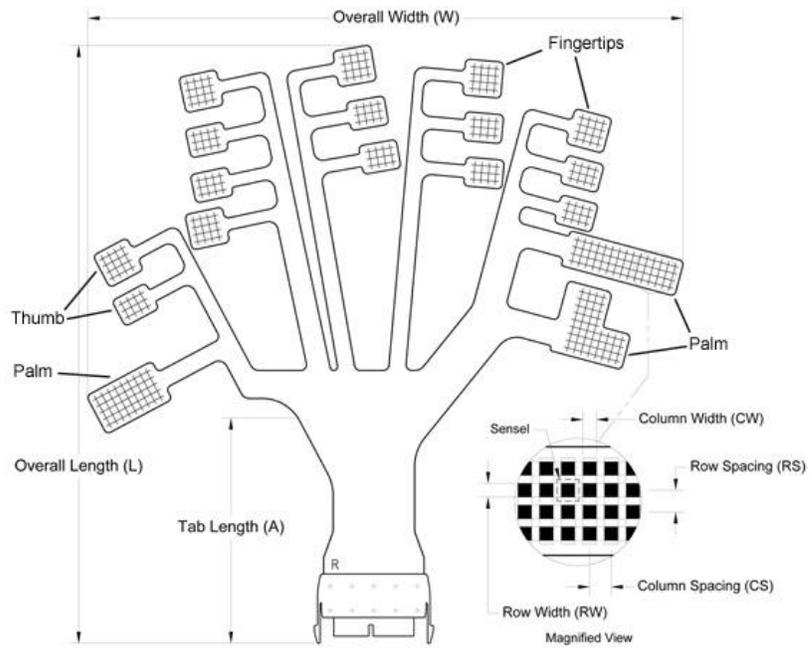
**Figure 5:** Location of the Sensors after attachment to a glove [30]
