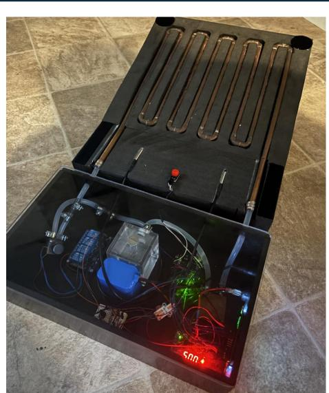
Housing for electronics and watercooling system. With temperature sensors, water tube and occupancy detector threaded through. 15mm R400H Velcrosecured down.
