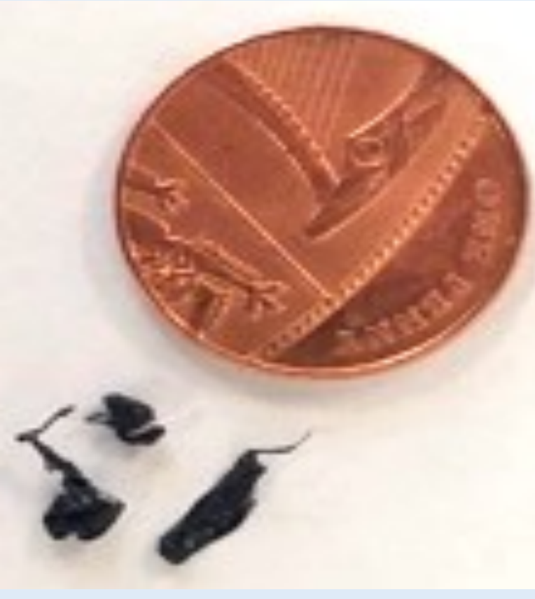
Figure 4: Debris size in print head
