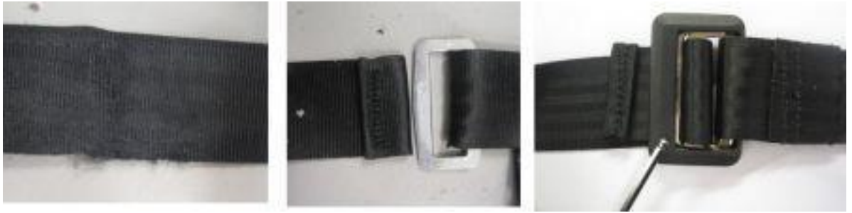
Figure 7.4.4: Post test webbing of pelvic belt (left and centre). Pre-test webbing (right)
