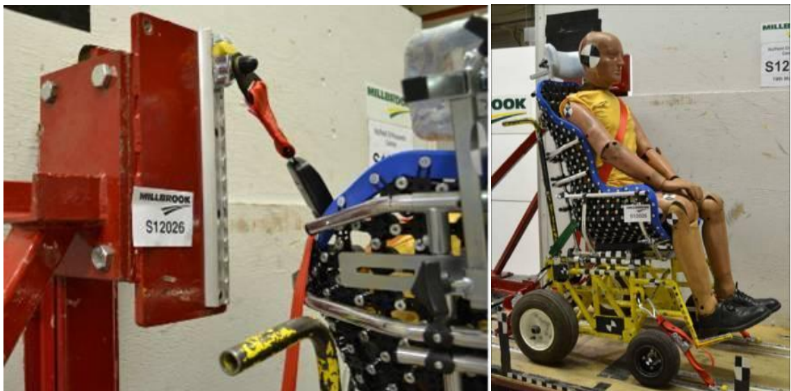
Figure 4.3: Set up of wheelchair integrated lap-belt with vehicle mounted torso belt and above shoulder vehicle mounted routing
