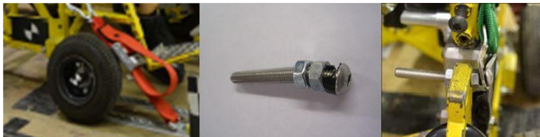
Figure 7.5.5: Deformation in front castor and anchor bolt
