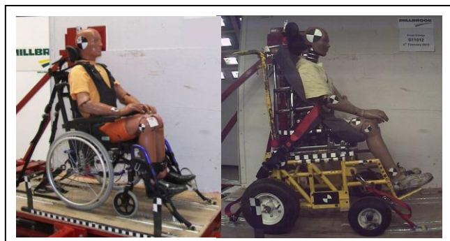
Figure 3.5.1: Seat tested with designated wheelbase (Left) and on surrogate wheelbase (Right)
