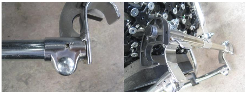
Figure 5.5: Interface with split pin (left) and mild steel cams behind nylon cams (right).
