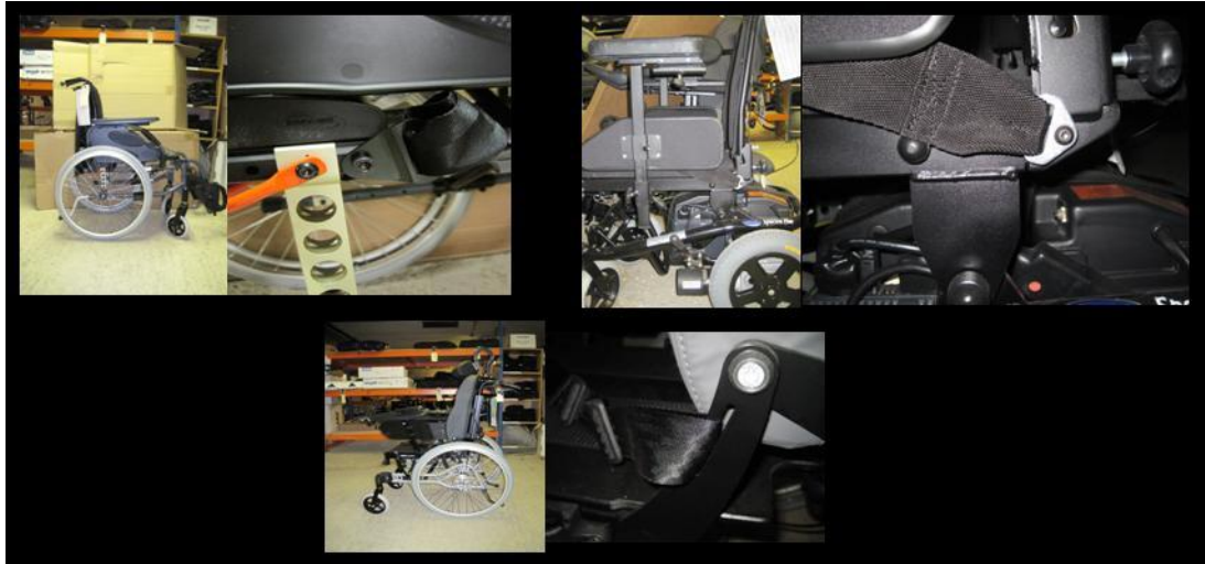
Figure 3.3.4: Invacare wheelchairs (Invacare UK Ltd, 2011) meet WC19 expectations with anchorage points. The Rea Azalia has a “loop around” arrangement (bottom right photograph)
