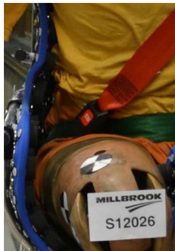
Figure 7.5.2: Torso belt found to be unfastened at the end of the test.
