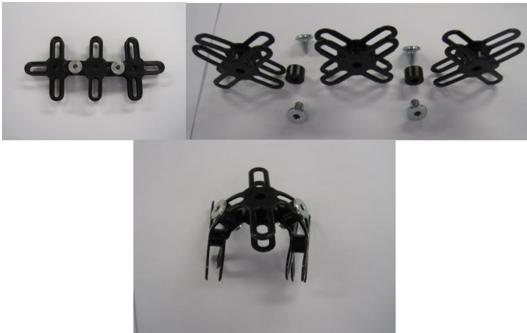
Figure 5.1: Lynx elements are used to create a shape-able Lynx sheet.
