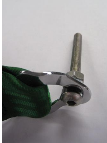
Figure 4.2: M8 stainless steel bolt with nylon bearing
