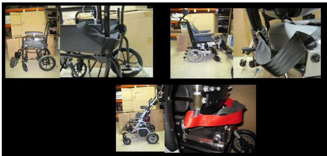
Figure 3.3.3: Simple "loop around" anchorages found on CAPS II seats (Active Design, 2011) and the Lomax range (Sunrise Medical UK Ltd, 2011)
