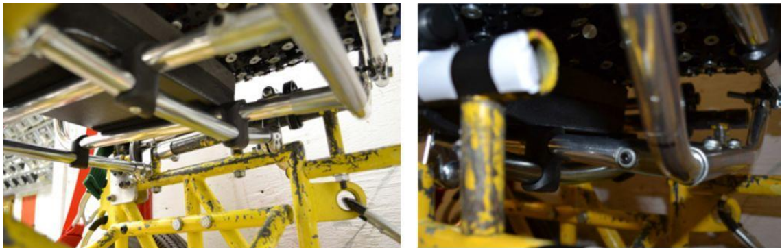
Figure 7.5.4: Some plastic deformation in cross member underneath front of seating system.
