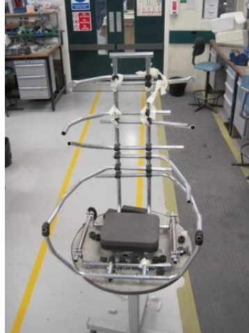
Figure 5.4: Mild steel sleeved uprights with aluminium framework tubing connected by nylon “X Joints”. Lynx seat rests on evazote base pad
