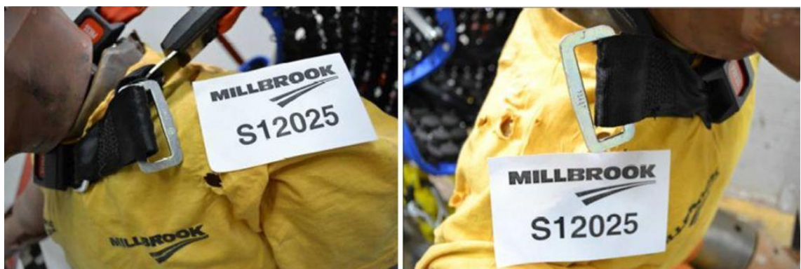
Figure 7.4.3: Detail of failure of pelvic belt restraint
