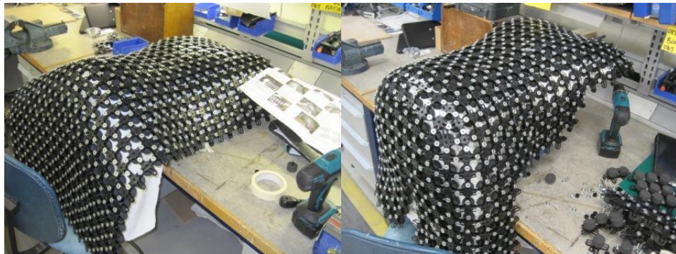
Figure 5.3: Pre tightened Lynx sheet laid over plaster cast.
