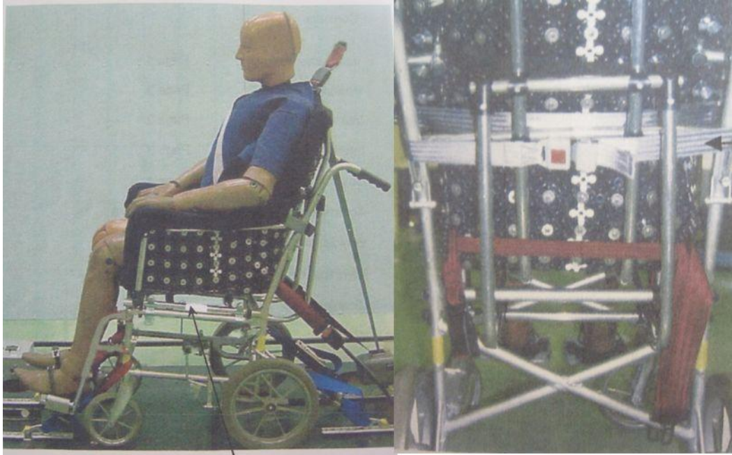
Figure 3.3.5: C & S seating from June 2001 with vehicle mounted pelvic belt and diagonal torso belt with vehicle mounted routing
