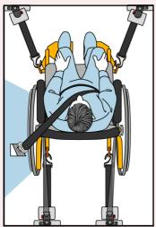
Front and rear tie-downs must be fitted to provide a stable seat for the wheelchair occupant.
