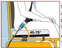
The lap belt should run at a steep angle, when viewed from the side, to maintain position and prevent the webbing applying load to the abdomen during a crash event.
