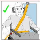
The lap belt must be routed under arm supports and side guards to achieve close contact with the pelvis of the wheelchair seated passenger.
