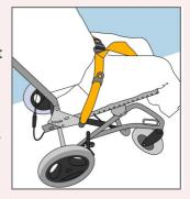
Wheelchair mounted head supports provide occupant comfort whilst in transport. Head supports should be positioned level with the occupant's head centre of gravity—approximately level with the passenger's ears.
