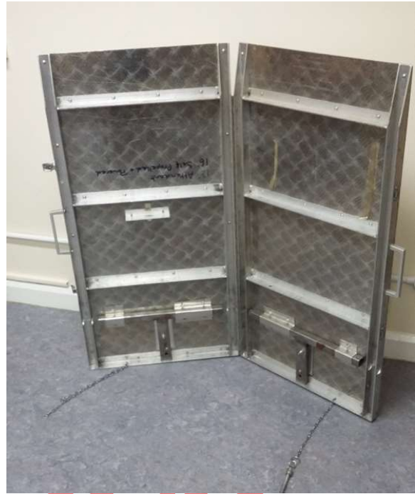
Figure 6 - Portable, folding, angle adjustable ramp - folding ramp
