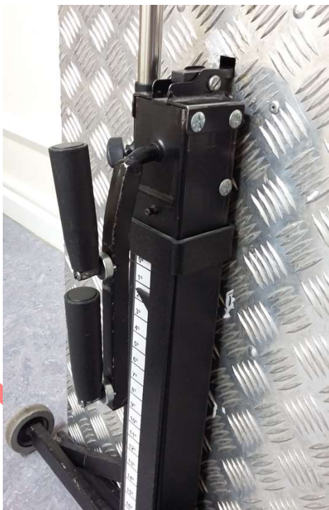
Figure 7 - Portable, folding, angle adjustable ramp - lifting jack with stored ramp
