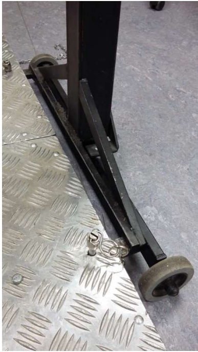
Figure 5 - Portable, folding, angle adjustable ramp - lifting jack fixation point
