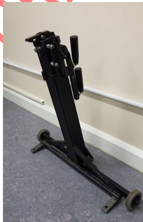
Figure 8 - Portable, folding, angle adjustable ramp - lifting jack
