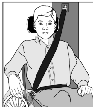
Figure 4. Good fit of a lap/shoulder belt system (Illustration courtesy of University of Michigan, used with permission)
